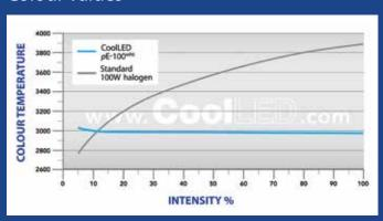
Correlated colour temperature (CCT) and colour rendering index (CRI) values are shown below. The  $pE-100^{wht}$  has been designed to match the standard settings of the 100W halogen lamp.
