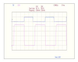
Independent control: Each color operates independently On/Off switching: Trigger via TTL, RS232, USB Intensity control: Choice of RS232, USB Switching rates: Up to 5 kHz Fast rise and fall times:  $t_{rise} < 10 \ \mu s$ ,  $t_{fall} < 5 \ \mu s$
