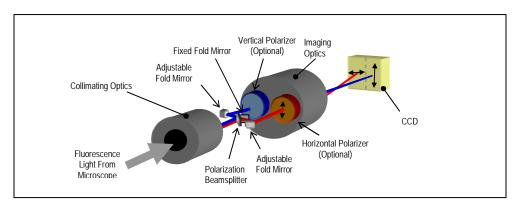
Figure 2: Operation of Dual-View™ fluorescence polarization imaging system.
